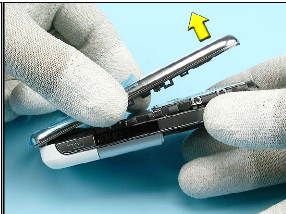
10. Remove the A-COVER and protect the inner window with a protective film.
