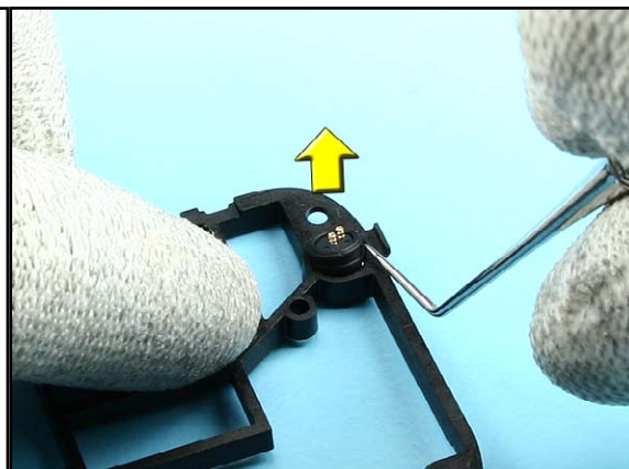
24. Remove the MICROPHONE CLAPTON with the dental pick.
