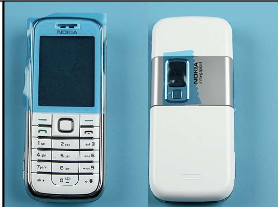
2. Protect the window with a protective film.
