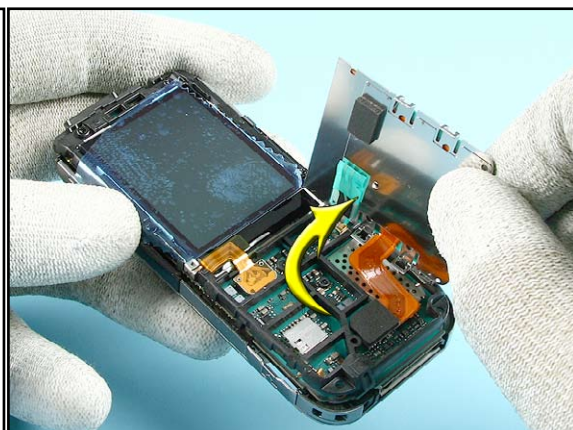
18. Flip over the C-COVER PLATE ASSY and pay attention to the flex foil.
