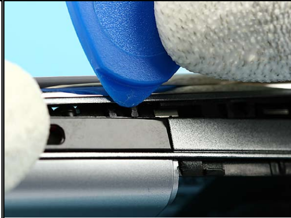
8. Bring the SRT-6 exactly to the position over the (invisible) clips. NOTE! A little sliding motion could be needed (like a 'credit card') when releasing the snaps. Do not damage the edges of the A-COVER.
